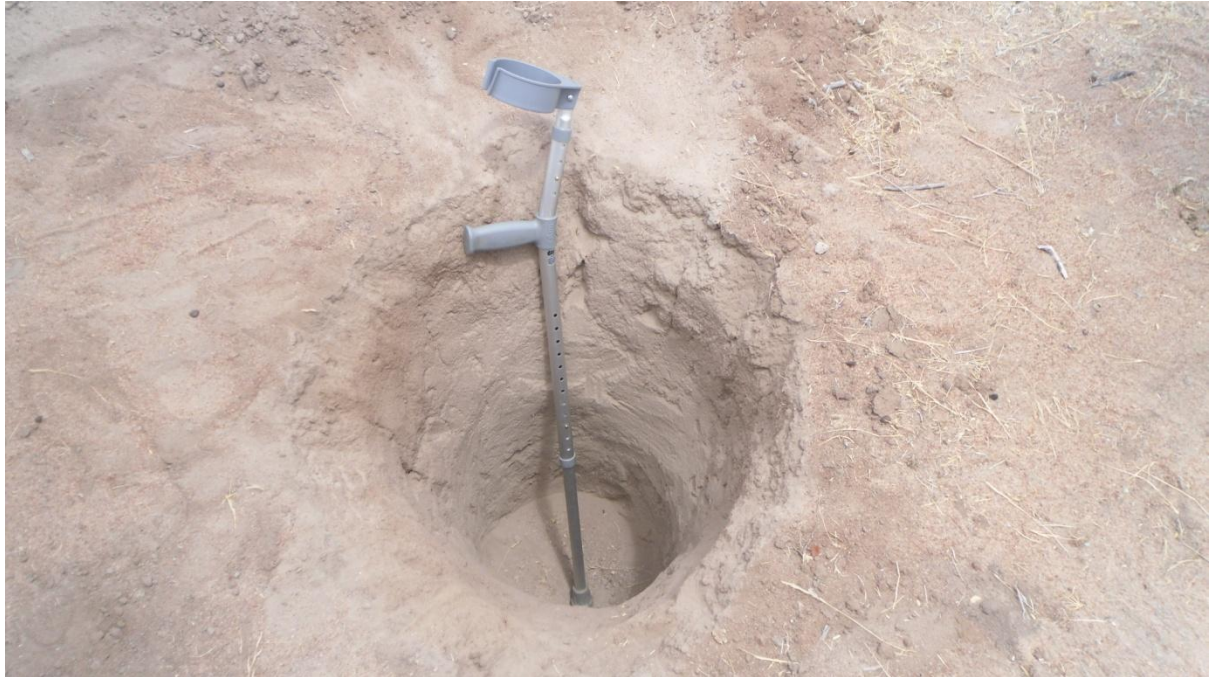
Figure 13: Pit excavated to study the soil profile on the proposed site
